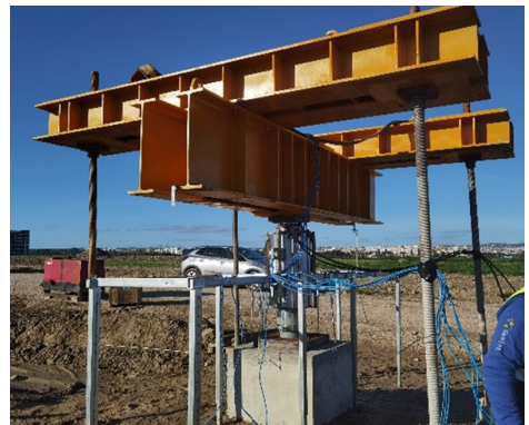
Figure 8 Reaction structure for the compression full scale load test
