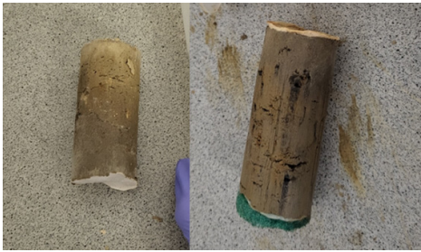
Figure 2-2 MICP treated samples after being removed from the tube, discolouration visible at the top showing a change in colour at the surface. Left B4 treated sample after 21 days. Right Deionised water treated sample after 21 days
