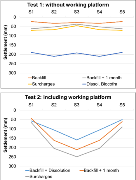
Figure 5 Settlement of the treated LTP
